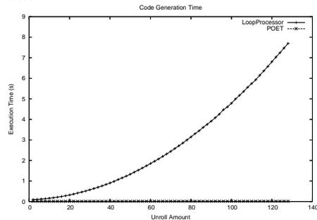
Fig. 8. Code generation time for different unroll factors
