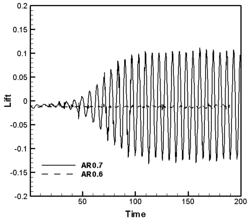
Figure 5. Lift Coefficient for ellipse (hydraulic diameter 1.0)
