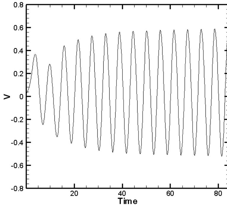
Figure 12. Lift Coefficient for Bottom Cylinder in FlowField
