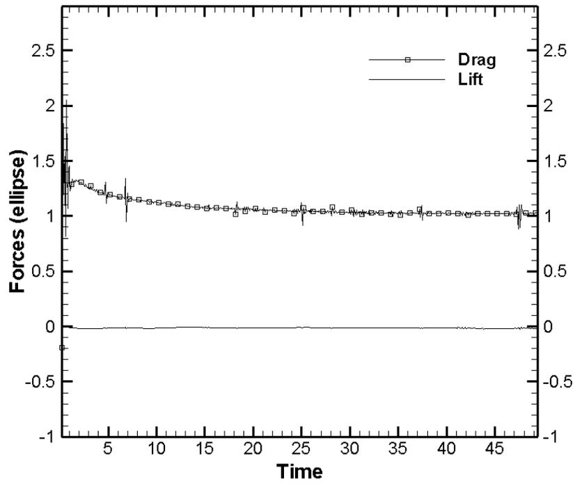
Figure 16. Drag and lift flow past an ellipse in 3D
