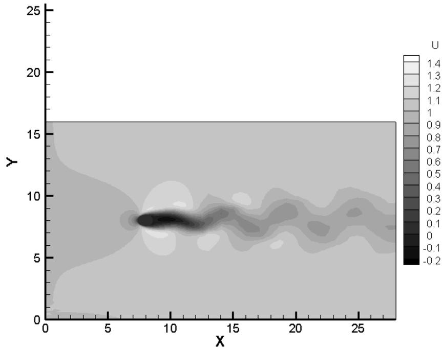
(a)  $U$  Contour
