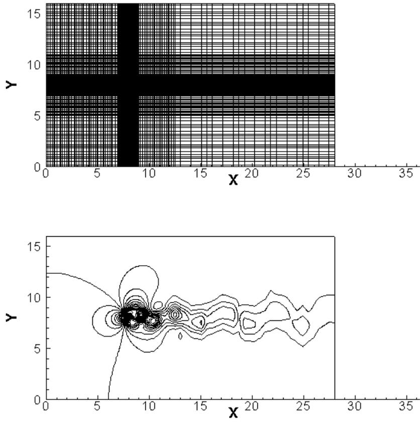
Figure 1. Re-200 Mesh and pressure contour plot (t-100)
