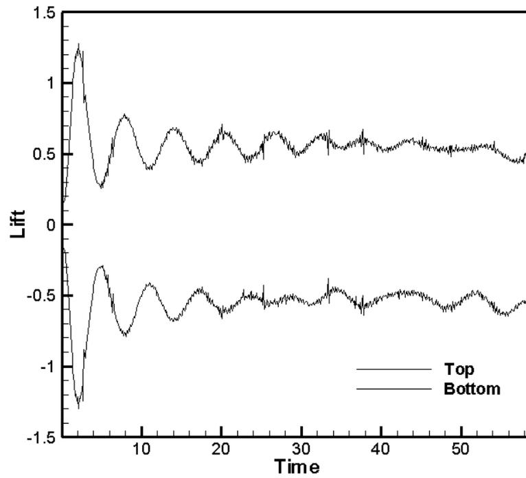
Figure 10. Lift Coefficient for two ellipses in flow field
