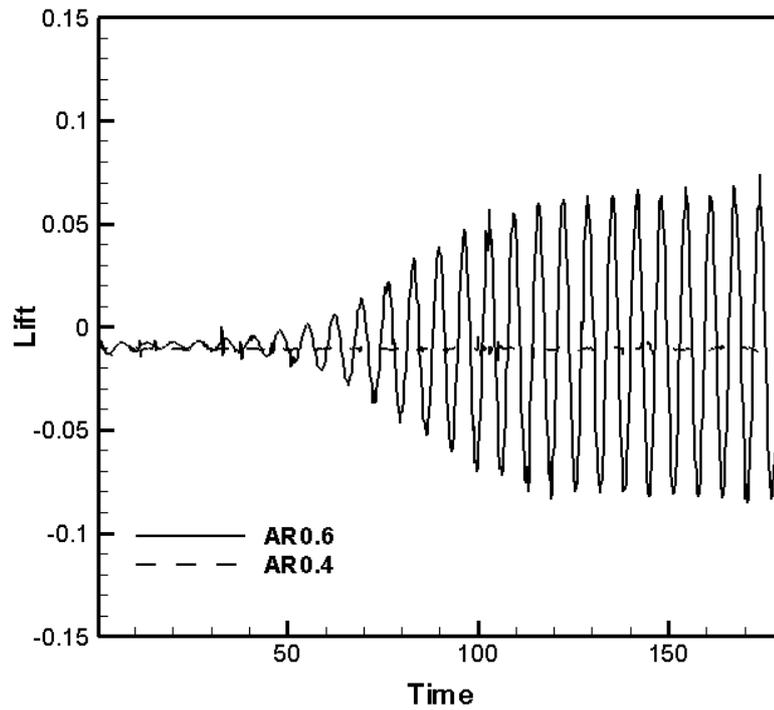
Figure 6. Lift Coefficient for ellipse in free stream
