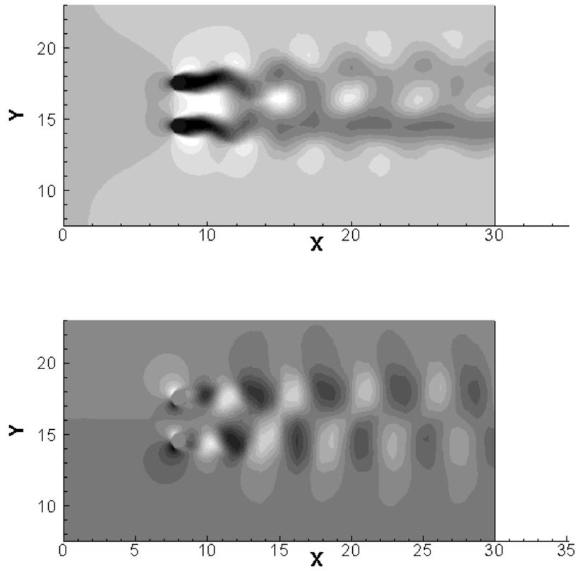
Figure 11. u-velocity and v-velocity contour plots  $S/D=2$
